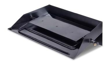
The Custom Embers Burner is a tapered wedge shaped burner that brings the front of the pan (and embers and flame) to the hearth level. It can be installed flush on the firebox floor, or elevated at the rear using the supplied rear height adjustment leg. The Custom Embers Burner is available in the following sizes:
