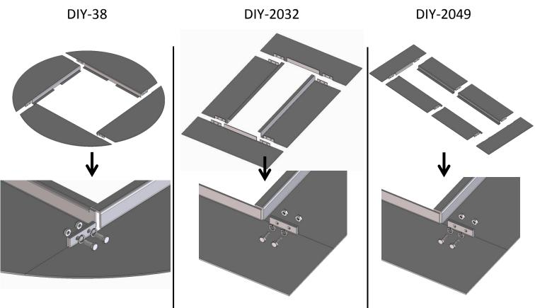
Step 2: Installing the Control Panel (suggested method for common cases)
