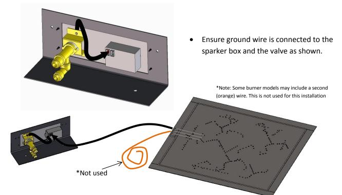
• Plug the **black** sparker wire into the igniter box. <u>A sparker wire extender is</u> included in your kit if the burner's wire does not reach your control panel location.
