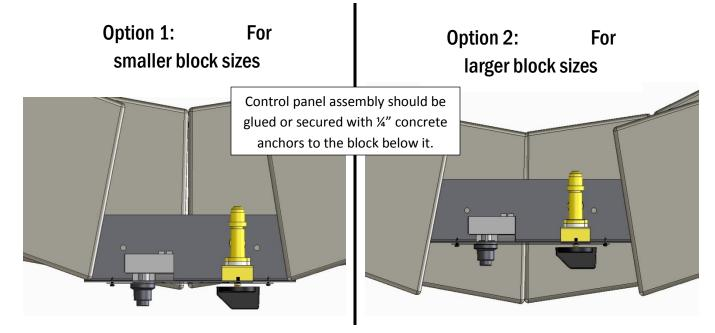
• For rectangular DIY fire pits, blocks should be cut to size for proper fit. Alternatively, mesh screen or other material can be cut and attached to control panel to act as filler around control panel.
