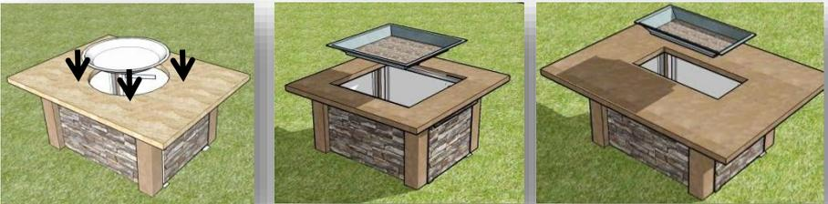
Lower burner onto base **with burner neck facing in the direction of control panel location.**
