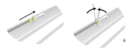
3. Set the burner into the fire pit table exactly as shown.
