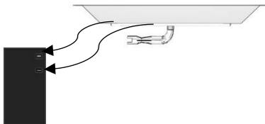
**After installing igniter and making gas connections, verify that gas connections are tight and that no leaks are present using a solution of soapy water or a commercially available leak-check solution.**
