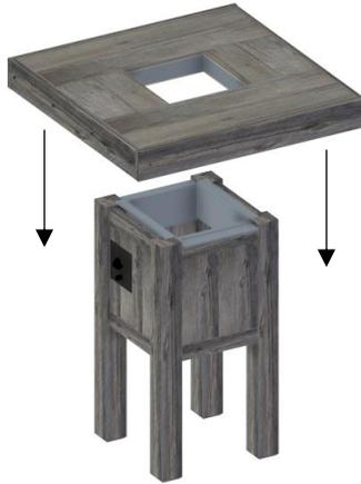
4. Using a power drill and **Self Tapping Philips Head Screws** provided, attach **Top Attachment Brackets** to secure **WP-TILETOP** to **WP-BASE** as shown in the figure below. Secure each attachment bracket using 4 screws.
