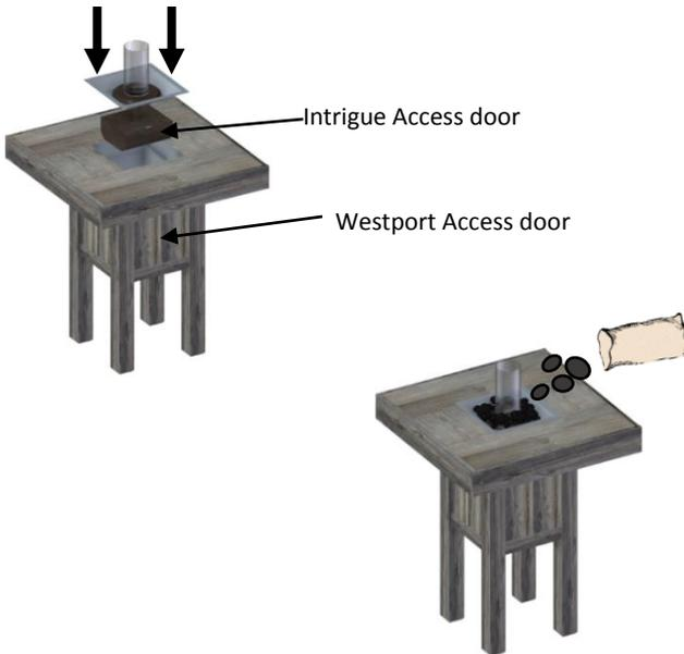
6. Carefully install tumbled lava rock; be careful not to damage the glass cylinder when installing lava rock.
