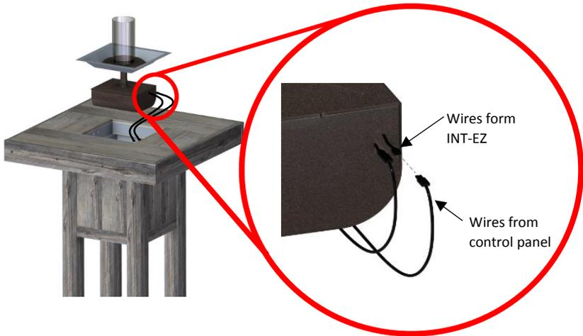
5. Drop INT-EZ and trim into fire pit. Orient the INT-EZ Base so that the access door is easily accessible.
