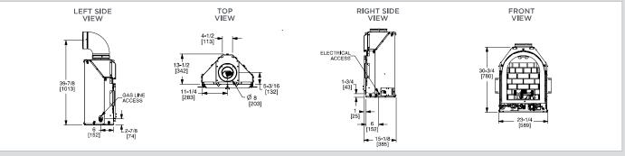
Dimensions above are in inches. Reference dimensions only, We recommend measuring individual units at installation, NOTE: Combustible material should not be installed over the face. Make sure you do NOT cover the decorative door opening.
